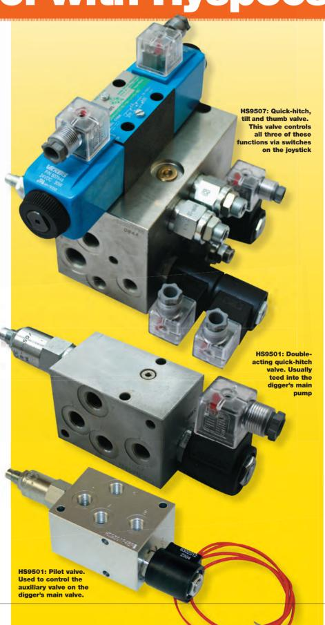
The first valves manufactured were designed to pilot-control the auxiliary valve on an excavator, or to directly control a single or double-acting quick-hitch cylinder. With the help of a hose installer, these valves can be quickly fitted to any new or old excavator.
